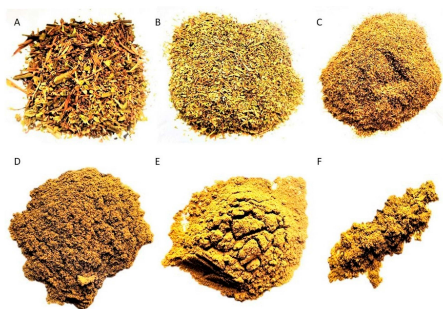
Figure 4. Nicotiana tabacum var. Virginia sieved fractions from ground inflorescence. (A) 840 \mu\text{m} . (B) 500 \mu\text{m} . (C) 149 \mu\text{m} . (D) 105 \mu\text{m} . (E) 74 \mu\text{m} . (F) less than 74 \mu\text{m} .
