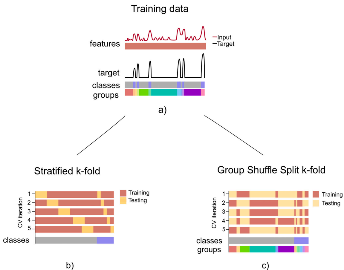
Fig. 4. Schematic representation of different k-fold cross-validation (CV) strategies. a) Training data, corresponding to an input vector of features (red) and an output target vector (black), e.g. movement trace, where two classes are involved and same sized groups are defined according to movement/no movement consecutive data chunks. b) In the standard stratified k-fold CV data is split into train and test sets, preserving class ratios in both sets. c) For invasive neurophysiological decoding we propose a group shuffled split k-fold CV strategy. While in the stratified k-fold CV class distributions are preserved along the CV iterations, features coming from the same group can be used for training and testing. The group k-fold CV ensures that group structure is preserved during training and testing set construction, but information about individual group blocks may not be preserved. For imbalanced class distributions data can either be rebalanced or cost function weights can be attributed class specific. (For interpretation of the references to colour in this figure legend, the reader is referred to the web version of this article.)
