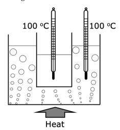
Figure 4. Internal vessel and external container filled with water. After enough heating and even when the temperature in both thermometers reaches the same value (boiling temperature), bubbles are only detected in the external container.
