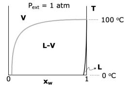
**Figure 3.** Projection of figure 1 on T-x<sub>w</sub> plane (not at scale).
