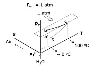
**Figure 1.**  $p_v$ -T- $x_{air}^L$  diagram (curve b-c is in the plane at P = 1 atm)
