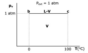
**Figure 2.** Projection of figure 1 on the p<sub>u</sub>-T plane
