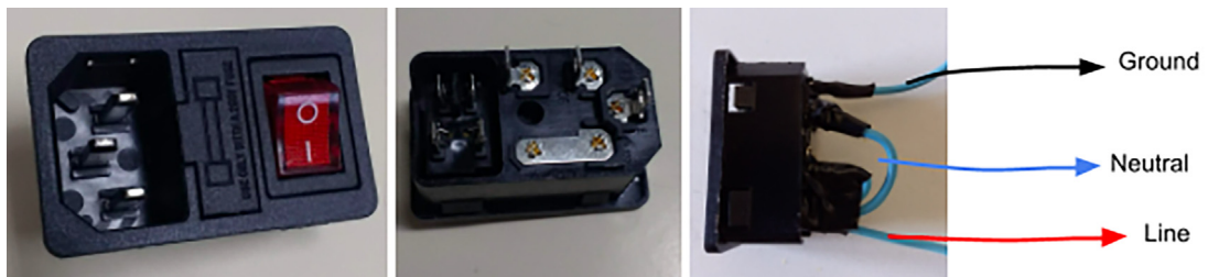
Fig. 10. Front view of the Fuse Switch (left), rear view (middle) and side view (right).
