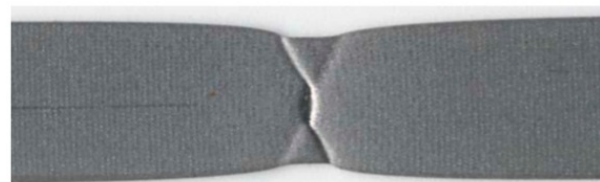
Figure 5. Fracture stage of an EK4 steel tensile sample.
