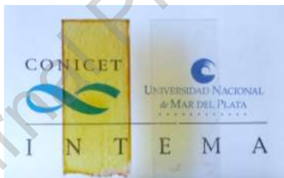
Figure 7. Photograph of TGL-Ag samples on glass substrates: original sample ( left ) and leached sample for 80 days ( right ).
