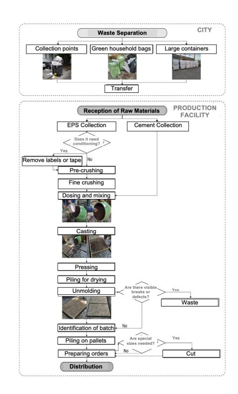
Figure 1. Flow diagram of the alternative thermal insulation board production process. Source: Preparation by the authors.
