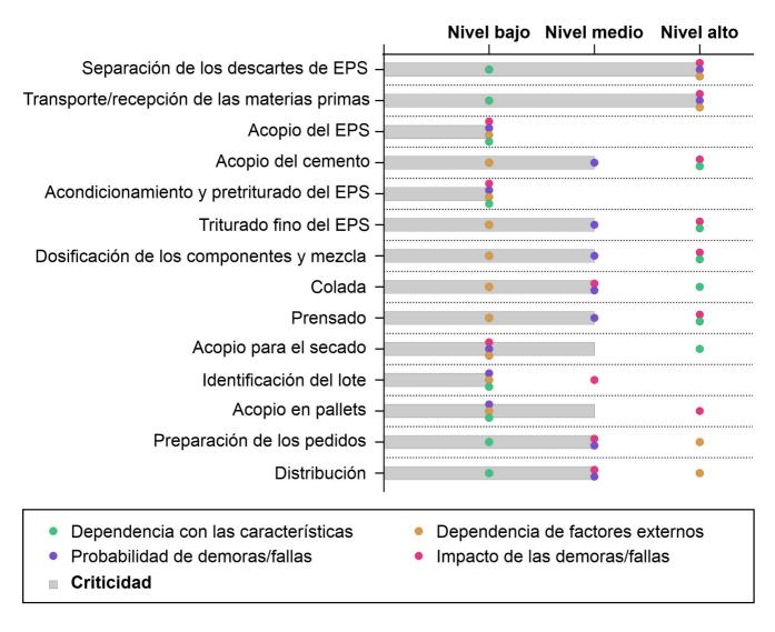
Figure 4. Level of criticality of the processes involved in the manufacture of alternative thermal insulation plates. Source: Preparation by the authors.
