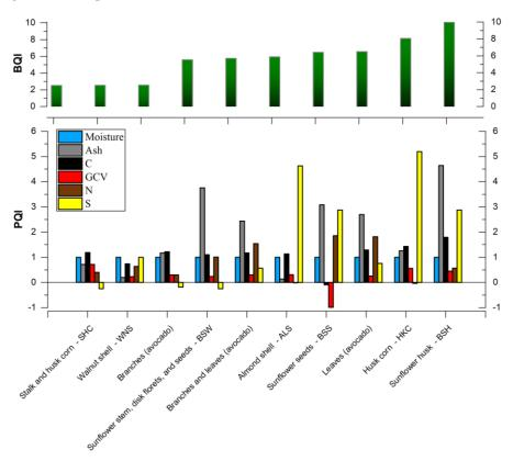
**Figure 1.** BQI ranking at fixed moisture content values (10%) for avocado pruning biomass and reference indices taken from [23].
