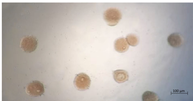
Figure 1. Optical microscopy image of microcapsules obtained by emulsification/rennet-catalyzed gelation of milk proteins (100× magnification).
