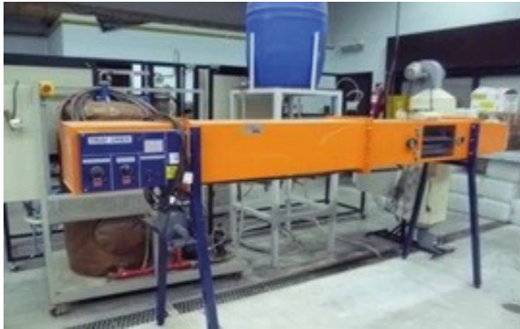
Figure 2. Experimental dryer (Armfield Tray Dryer Type UOP8-A, Armfield Ltd Ringwood, Hampshire, UK) and scheme from original Armfield catalogue (1997)
