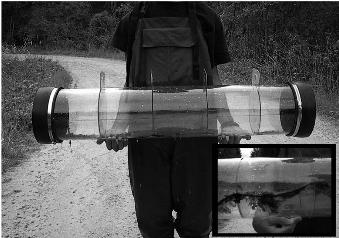
Fig. 2. Sampling device for mixed-mat floating macrophyte community, showing typical sample material.
