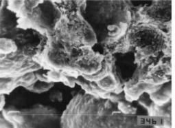
Figure 1: Left: Lamellar zinc dust (SEM, 1000x); Right: lamellar zinc primer film (SEM 7500x; 1200 hr salt fog chamber)
