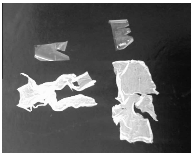
Fig. 2. Shows a picture of two pairs of samples in which the smaller ones are the original substrata and the larger ones the grafted replicas. The experimental parameters were 79% AAC, 0.2 M sulfuric acid in aqueous solution, 22 h grafting time, 10^{13} cm -2 ion fluence and 100 keV ion energy.
