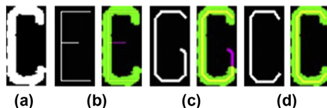
Fig. 5. Example of segmented letter (a), superimpose with incorrect skeletons (b) (c) and the correct one (d).
