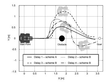
Fig. 11. Trajectories followed by the remote mobile robot using the scheme B.
