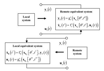
Fig. 3. Local and remote equivalent systems.
