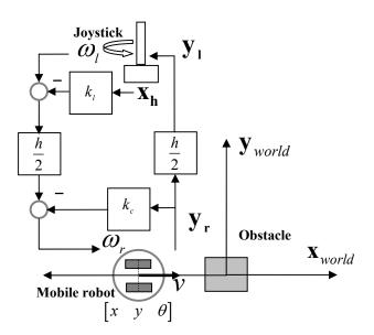
Fig. 6. Teleoperation system of a mobile robot with force feedback.
