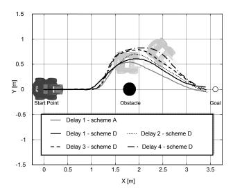
Fig. 13. Trajectories followed by the mobile robot using the scheme D.
