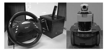
Fig. 9. Mobile robot teleoperated through a joystick with force feedback and steering wheel.
