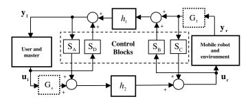
Fig. 7. General control schemes for bilateral teleoperation of mobile robots.
