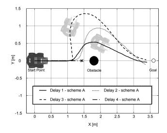
Fig. 10. Trajectories followed by the remote mobile robot using the scheme A.
