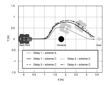
Fig. 12. Trajectories followed by the remote mobile robot using the scheme C.
