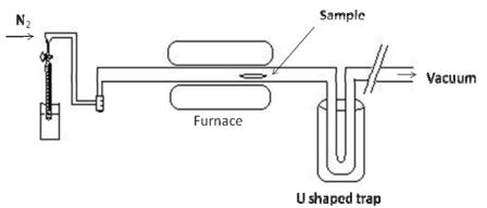
Figure 1. Schematic diagram of pyrolysis system
