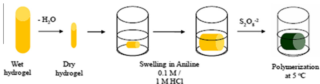
Scheme 3. Sequence of steps used to semi-interpenetrate a polyaniline into the hydrogel.
