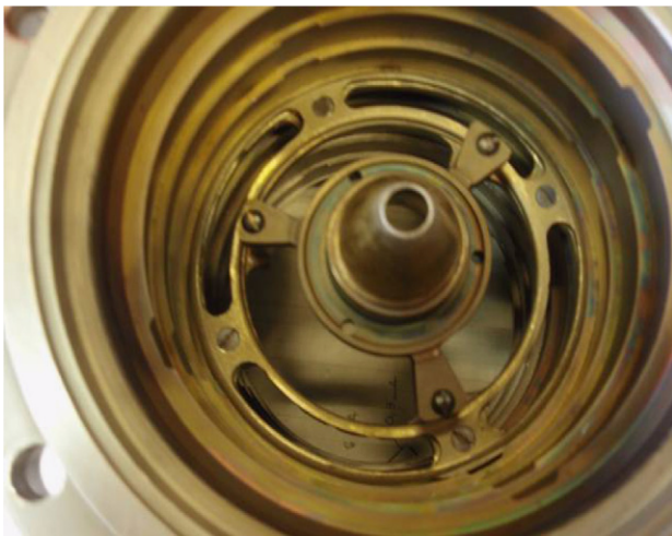
Fig. 7. First extraction electrode within acceleration tube (pointing towards the ion source).
