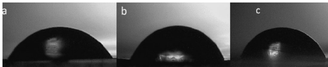
Fig. 5. Photographies of water drop onto PPy nonstructured (a), and structured PPy with lines pattern (0.9 \mu\text{m} wide) (b) and (c) PPy with grid pattern,(period 3.5 \mu\text{m} ).
