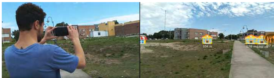
Fig. 1: ARPOT in use. The icons are always fixed in the corresponding place, even when the user walks and rotates. A small label also shows the distance between the user and the point-of-interest. (Left) Student looking for a particular point-of-interest. (Right) Device view.
