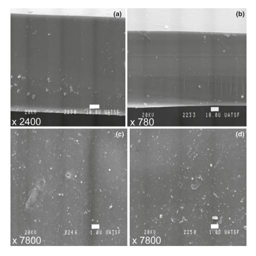
Figure 4. Morphology of cross-sections (**a** and **b**) and surfaces (**c** and **d**) of cross-linked membranes prepared from a concentration of chitosan of 2.66% w/v (**a** and **c**) and 3.5% w/v (**b** and **d**).
