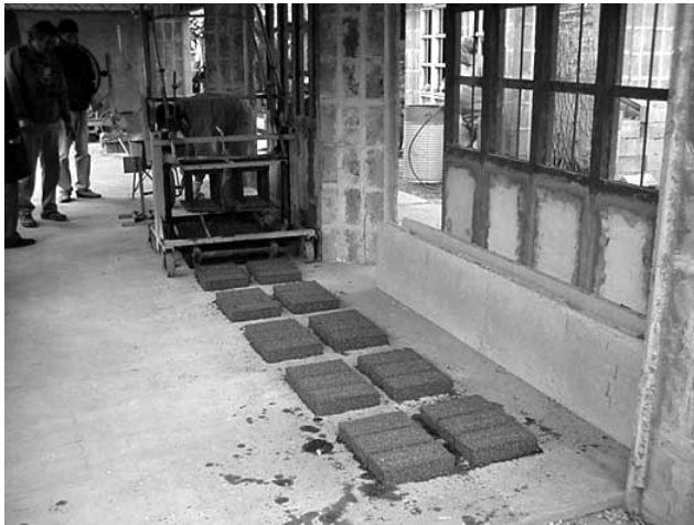
Fig. (4). Machine used to make bricks with recycled plastics.
