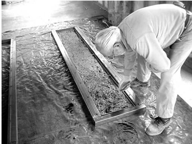
Fig. (8). Monolithic slab made of recycled plastics.
