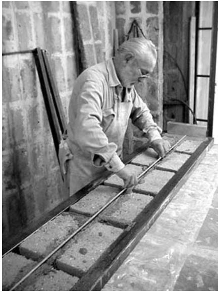
Fig. (7). Bricks slab made of recycled plastics.
