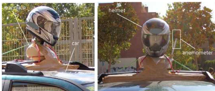
Fig. 5. Experimental setup for the freeway experience. The mannikin and the helmet with the microphones and the anemometer were located in the car's roof.
