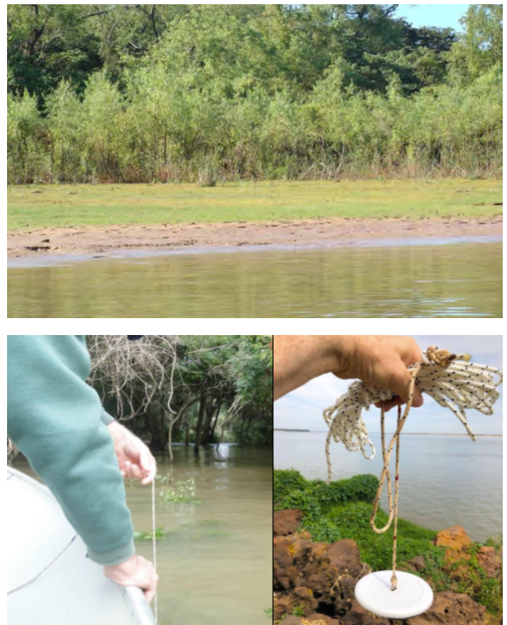
FIGURE 4. Measurement of the topographical position of a floodplain point during high water (left picture) with a metal disc (“scandal”), placed at the end of a thin cord which is graduated every 10 cm (right picture).
