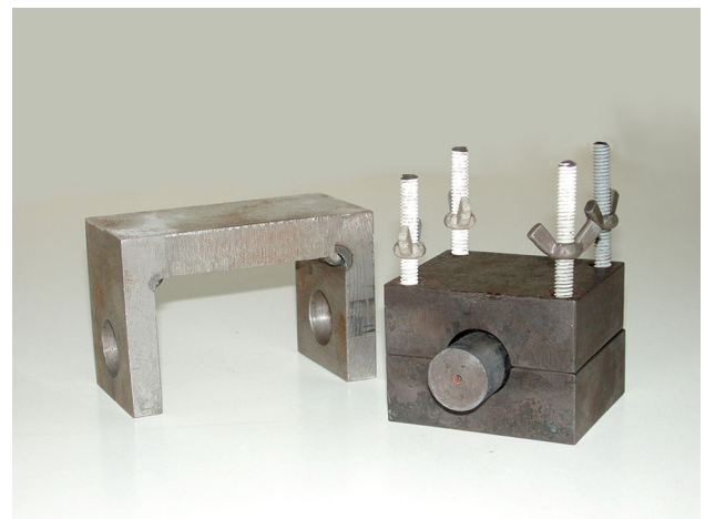
Fig. 10 Photograph of the compound bending die
