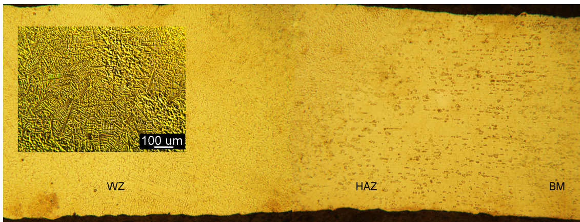
Fig. 3 OM image of the microstructure of the welded sheet: welded zone (WZ), heat-affected zone (HAZ), base metal (BM). The inset shows the cellular-dendritic structure in the WZ
