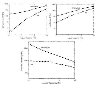
Fig. 4. Rheological properties of PP and PP/MWCNT.
