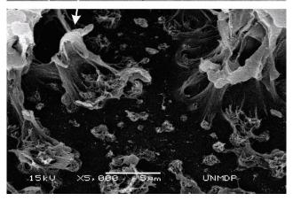
Fig. 6. SEM of post morten fracture surfaces of PP/MWCNT tested under flexural load.
