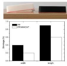
**Fig. 2.** Boxes aesthetic characteristics: lateral view of injected boxes and their shrinkage.
