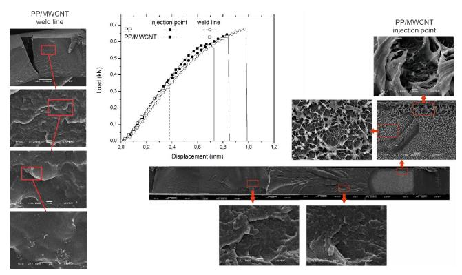
Fig. 7. Typical load-displacement curves for PP and PP/MWCNT samples obtained from different places of the injected pieces and fracture surfaces of PP/MWCNT samples observed by SEM.
