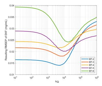
**Figure 7.** Error in the EKF prediction of the monoclonal antibody (mAb) concentration as a function of the model mismatch factor  $k_O$  for each of the BT curves of the calibration set of ROT1.
