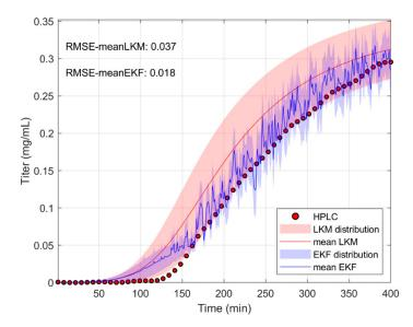
**Figure 8.** Effect of 5% Gaussian distributed perturbations in feed concentration and flow rate, as well as bed porosity on the predictions of the LKM (mean = dark red; standard deviation interval = light red) and the EKF (mean = dark blue; standard deviation interval = light blue) of ROT1 in 200 simulations.
