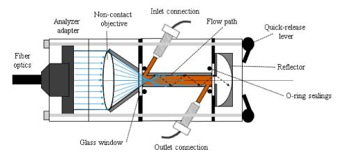
Figure 1. Schematic illustration of the developed flow cell.
