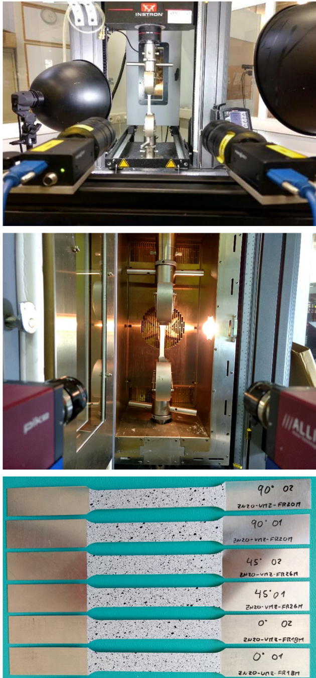
Fig. 1 – Top: Strain-rate setup. Middle: The heating chamber for variable temperature experiments. Bottom: ASTM E8 Tensile test samples with speckle pattern.
