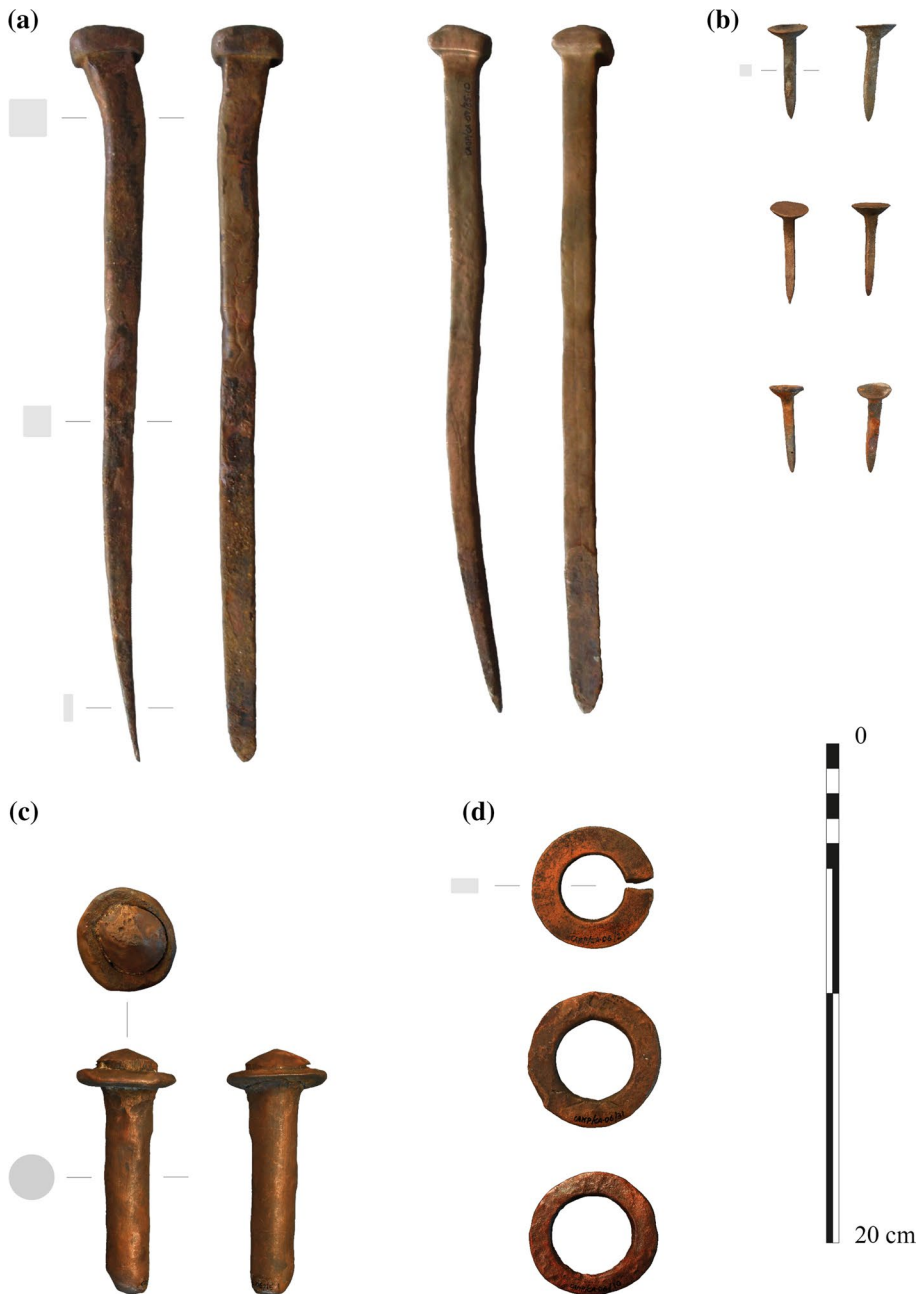
Fig. 1 Copper-based fastenings from the French shipwreck Fougueux (1805): a front and right side view of two spikes; b sheathing tacks; c front, top, and right side view of a bolt with clinch ring; and d clinch rings (after Ciarlo 2016). Courtesy of the Centre for Underwater Archeology of the Andalusian Historical Heritage Institute (CAS-IAPH)
