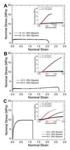
**Figure 4.** Stress–strain curves of water kefir films with different content of glycerol. Formulations K1.5, K3, and K5 were obtained from film-forming dispersion of (**A**) 1.5, (**B**) 3, and (**C**) 5 wt% dry matter of water kefir grains, respectively.
