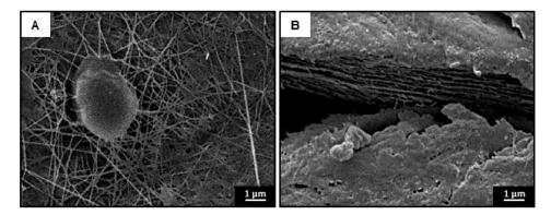
**Figure 6.** SEM observations of the dried Kombucha cellulose surface at 7000× magnification (**A**) and cross-sections (7000×) (**B**) of cellulose film.
