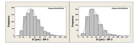
Figure 10. The distribution of initial average size  $D_0$  for two samples of the pure ZA27 alloy at 460°C during 15 minutes.
