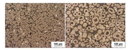
Figure 14. Coalescence of pure ZA27 alloys during the heat treatment (a) 15 min and (b) 45 min.
