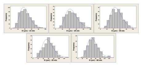
Figure 13. Particle size frequency distribution of the ZA27-2%Cu-0.015%Mg alloy during the heat treatment. Adjusted to Gamma distribution.
