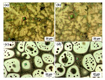
**Figure 15.** Microhardness of the as-cast of ZA27 pure alloy before and after the SIMA process applied: a) indentation of the dendrite score, (b) indentation of the interdendritic region, (c) indentation of the globular phase and (d) indentation of the interglobular phase.
