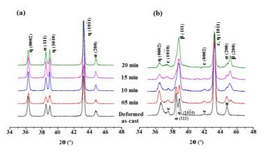
Figure 6. X-ray diffractograms of the deformed sample of the alloys during partial remelting at semi-solid temperature of 460 °C: (a) ZA27 and (b) ZA27-2%Cu-0.015%Mg.
