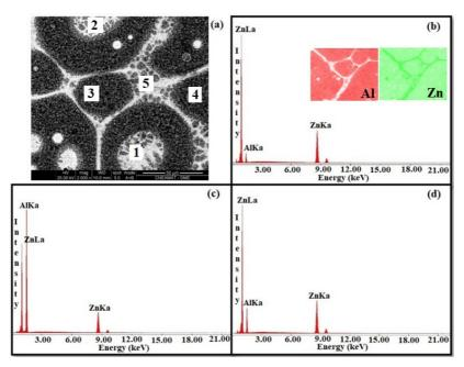
**Figure 7.** SEM images of ZA27 alloys during 20 min at 460 °C: (a) the pure ZA27 alloy with the measuring points by EDAX: (1-2) Intraglobular, (3-4) Globular and (5) Interglobular. (b) EDS spectra of interglobular zone with micrograph of mapping of elements, (c) EDS spectra of globular zone and (d) EDS spectra of intraglobular zone.
