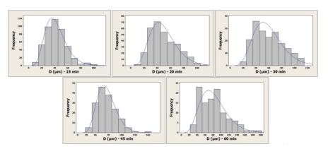
Figure 12. Particle size frequency distribution of the pure ZA27 alloy during the heat treatment. Adjusted to Gamma distribution.
