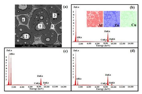
**Figure 8.** SEM images of ZA27 alloys during 20 min at 460 °C: (a) the ZA27 alloy contained Cu and Mg with the measuring points by EDAX: (1-2) Intraglobular, (3-4) Globular and (5) Interglobular. (b) EDS spectra of interglobular zone with micrograph of mapping of elements, (c) EDS spectra of globular zone and (d) EDS spectra of intraglobular zone.
