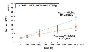
**Figure 11.** Relationship between  $(D_{t}^{3}-D_{0}^{3})$  of the grains versus the isothermal time treatment taking 15 min as initial time ( $t_{0}$ ).
