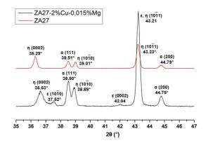
Figure 1. XRD pattern of as-cast ZA27 and ZA27-2%Cu-0.015%Mg alloys.
