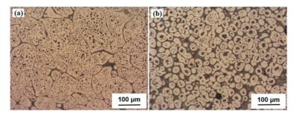
Figure 3. Optical microscope images of ZA27 pure alloys treated at 460 °C during 20 min and after deformed in thickness: (a) 10% and (b) 20%.
