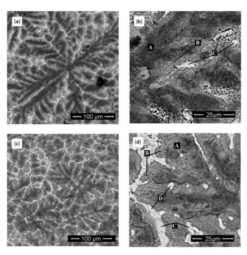
Figure 2. SEM micrographies of dendritic microstructure of the as-cast alloys: (a) and (b) ZA27 alloy; (c) and (d) ZA27-2%Cu-0.015%Mg alloy. Markers are explained in the main text.
