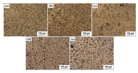
Figure 5. Optical micrographs of the microstructure of the deformed ZA27 alloy (a) when it is partial remelted for (b) 5 min, (c) 10 min, (d) 15 min, (e) 20 min at temperature of 460  $^{\circ}$ C and (d) 15 min.
