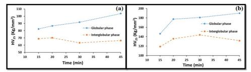
Figure 16. Microhardness of the ZA27 and the ZA27-2%Cu-0.015%Mg alloys, treated at 460°C with the heating time.
