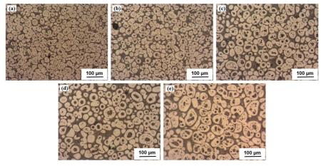
Figure 9. Evolution of phases and species distribution of pure ZA27 alloys thermally treated at 460 °C at different time: (a) 15 min, (b) 20 min, (c) 30 min, (d) 45 min and (e) 60 min.
