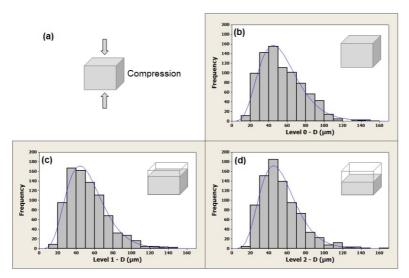
Figure 4. Distribution of grain sizes at different depths of pure ZA27 alloy: (a) The arrow indicates the compression direction, (b) level 0 (surface), (c) level 1 (0.15 cm below surface) and (d) level 2 (0.30 cm below surface).
