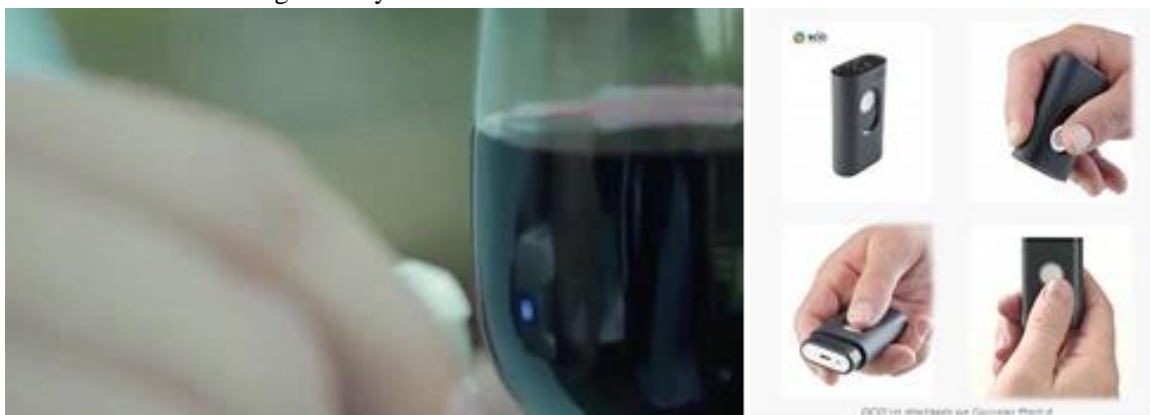
Fig. 1 SCIO® molecular sensor measuring the antioxidant activity of wine in a glass.
