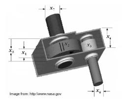
Figure 3: Speed Reducer.
