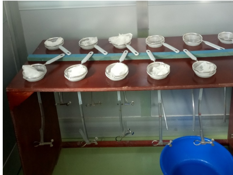
Fig 2. Funnel stand with Baermann apparatus for filtering of S. stercoralis larvae from stool samples.
