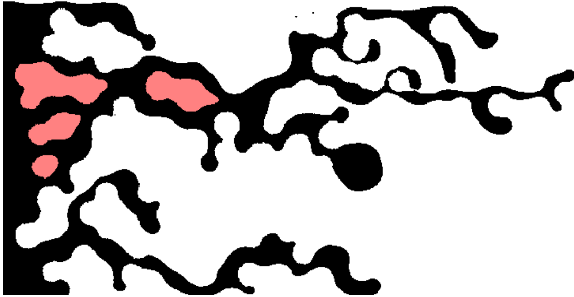
Figure 4. The entrapment effect in the micromodel. The flow direction is from left to right. White represents the porous medium, black is the displacing fluid, and red is the entrapped oil.
