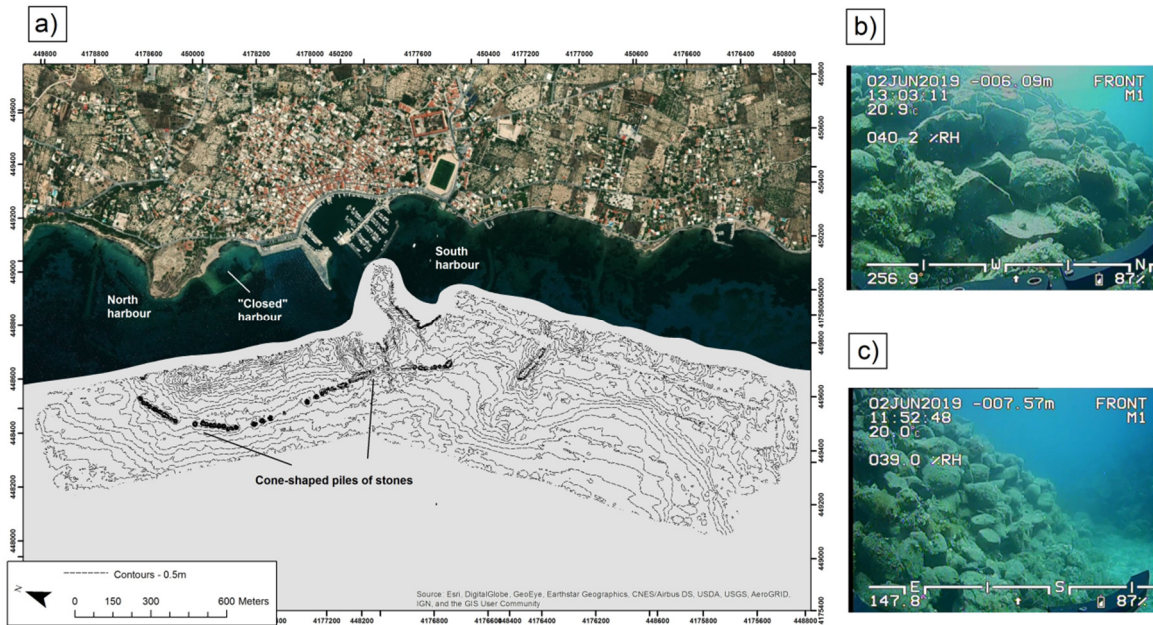
Figure 3. Detail bathymetric map of the ancient harbor of Aegina based on multibeam data (a) and underwater photos showing the cone-shaped piles constructed by stones, part of the submerged ancient harbor installations (b,c). Photo credits: University of Patras.
