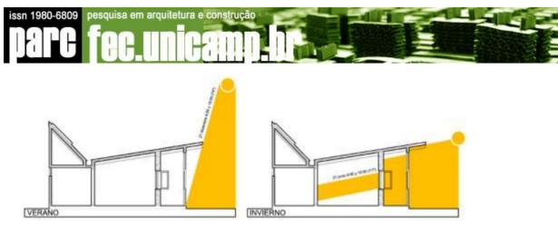
Figure 5 Solar gain an protection in the conservatory space
