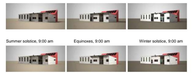
Summer solstice, 3:00 pm Equinoxes, 3:00 pm Winter solstice, 3:00 pm Figure 6 Solar gain studies on the north elevation
