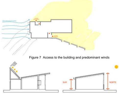
Figure 8 Roof slopes according to flat solar collectors and solar orientation
