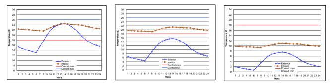
Figure 17 Indoor and outdoor temperature simulations in a day in January (left), October (center) and July (right)
