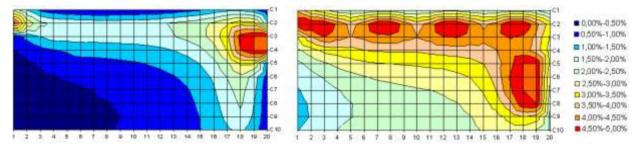
Figure 15 Daylight studies (Daylight Factor): initial simulations (left) and adpted model (right)
