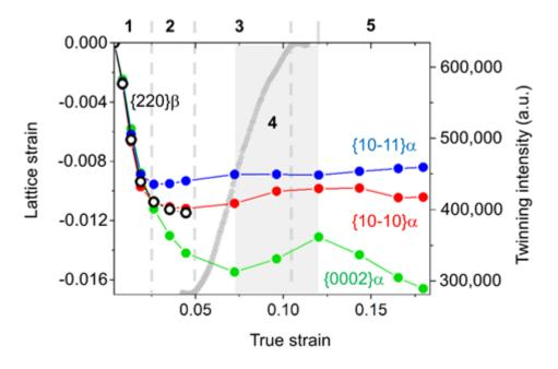
**Figure 4.** Deformation stages: 1) elastic regime, 2) slip activation, 3) twinning formation, 4) relaxation of the matrix (deformation dominated by twinning), 5) deformation dominated by slip. Evolution of the twinning intensity (grey curve) and lattice strains obtained for the hcp  $\{0002\}\alpha$ ,  $\{10-10\}\alpha$  and  $\{10-11\}\alpha$  planes, as well as for the bcc  $\{220\}\beta$  plane in the compression direction during deformation. The error bars are comprised within the symbols.
