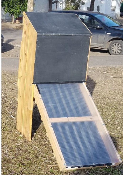
Figure 5: Experimental wood dryer
