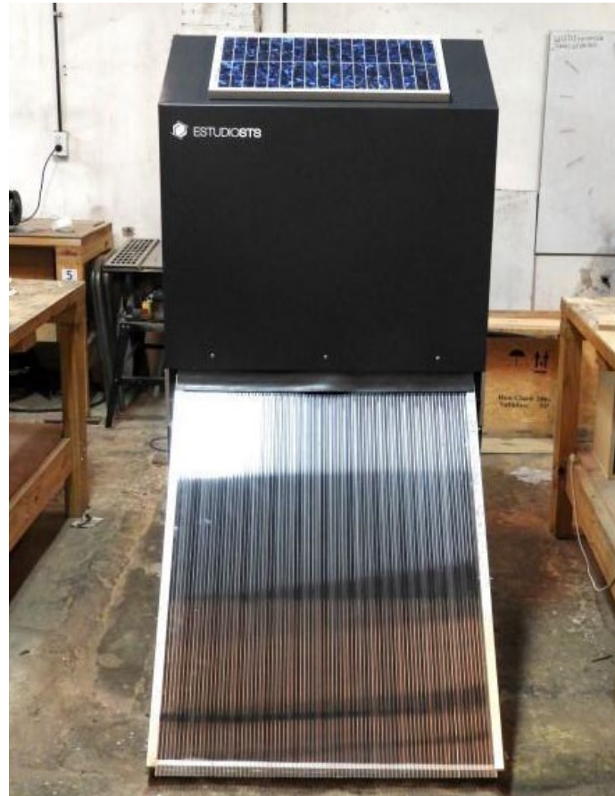
Figure 6: Metallic dryer for small producers
