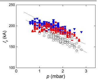
**Figure 4.** Pinch current dependence on the pressure. The data points corresponding to the configurations without any barred cathode are represented by empty circles (black), the data corresponding to discharges using a cathode of 41 mm radius is represented by down triangles (blue) and the discharges using the 45 mm radius cathode are represented by up triangles (red). Every point corresponds to a discharge that produced emissions of x-rays and neutrons.
