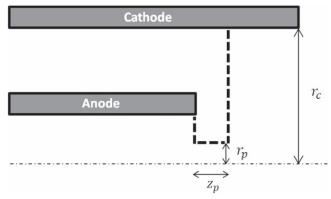
Figure 8. Simplified effective geometry of the radial collapse of the current sheath.
