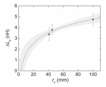
**Figure 9.** Inductance jump during the radial collapse,  $\Delta L_p$ , plotted as function of the cathode radius. In the case without barred cathode the chamber wall is taken as acting cathode.
