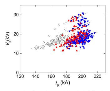
**Figure 6.** Voltage drop on the current sheath at the pinch time. The data points corresponding to the configurations without any barred cathode are represented by empty circles (black), the data corresponding to discharges using a cathode of 41 mm radius is represented by down triangles (blue) and the discharges using the 45 mm radius cathode are represented by up triangles (red). Every point corresponds to a discharge that produced emissions of x-rays and neutrons.
