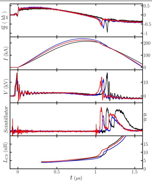
**Figure 2.** Comparison of typical signals of a single shot at 1.8 mbar utilizing the barred-cathode configuration of 45 mm radius (red) and 41 mm radius (blue), and without barred-cathode (black).
