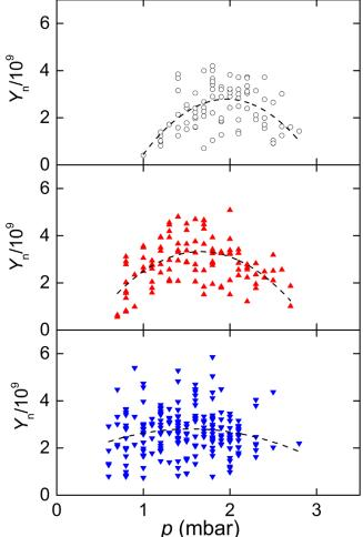
**Figure 10.** Neutron yield dependence on the pressure without any barred cathode (up), 41 mm radius barred cathode (middle) and 45 mm radius barred cathode (down).
