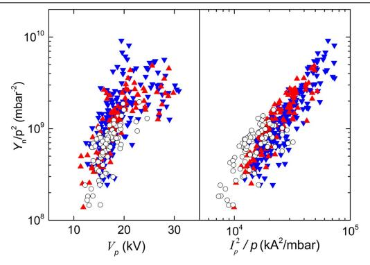
Figure 11. Reactivity of the pinch,  $Y_n/p^2$ , plotted against the voltage drop along the pinch  $V_p$  (left) and against  $I_p^2/p$  (right).
