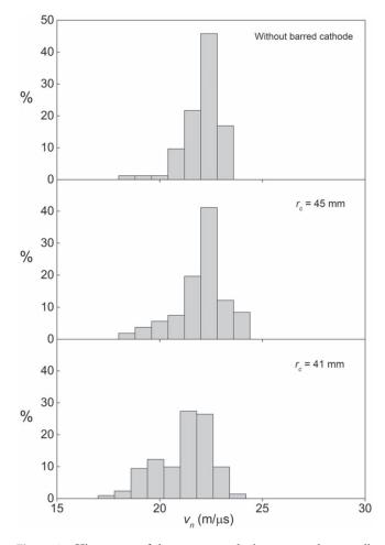
Figure 12. Histograms of the neutrons velocity measured perpendicularly to the pinch axis.
