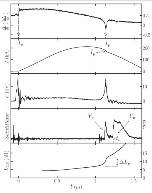
Figure 1. Typical signals of a single shot at 1.8 mbar utilizing the 45 mm radius barred cathode, showing the characteristic magnitudes extracted for analysis.
