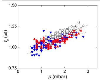
**Figure 3.** Pinch time dependence on the pressure. The data points corresponding to the configurations without any barred cathode are represented by empty circles (black), the data corresponding to discharges using a cathode of 41 mm radius is represented by down triangles (blue) and the discharges using the 45 mm radius cathode are represented by up triangles (red). Every point corresponds to a discharge that produced emissions of x-rays and neutrons.
