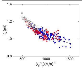
**Figure 5.** Pinch time as function of the parameter  $(I_p/r_a)\sqrt{\mu_o/p}$ . The data points corresponding to the configurations without any barred cathode are represented by empty circles (black), the data corresponding to discharges using a cathode of 41 mm radius is represented by down triangles (blue) and the discharges using the 45 mm radius cathode are represented by up triangles (red). Every point corresponds to a discharge that produced emissions of x-rays and neutrons.
