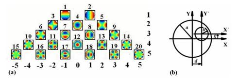
**Figure 1** (a) Zernike pyramid for  $j \le 20$ . (b) Pupil scaling and decentering, *a*: original pupil radius, *b*: new pupil radius, (d,g): pupil decentering  $(f=(d^2+g^2)^{1/2})$ .
