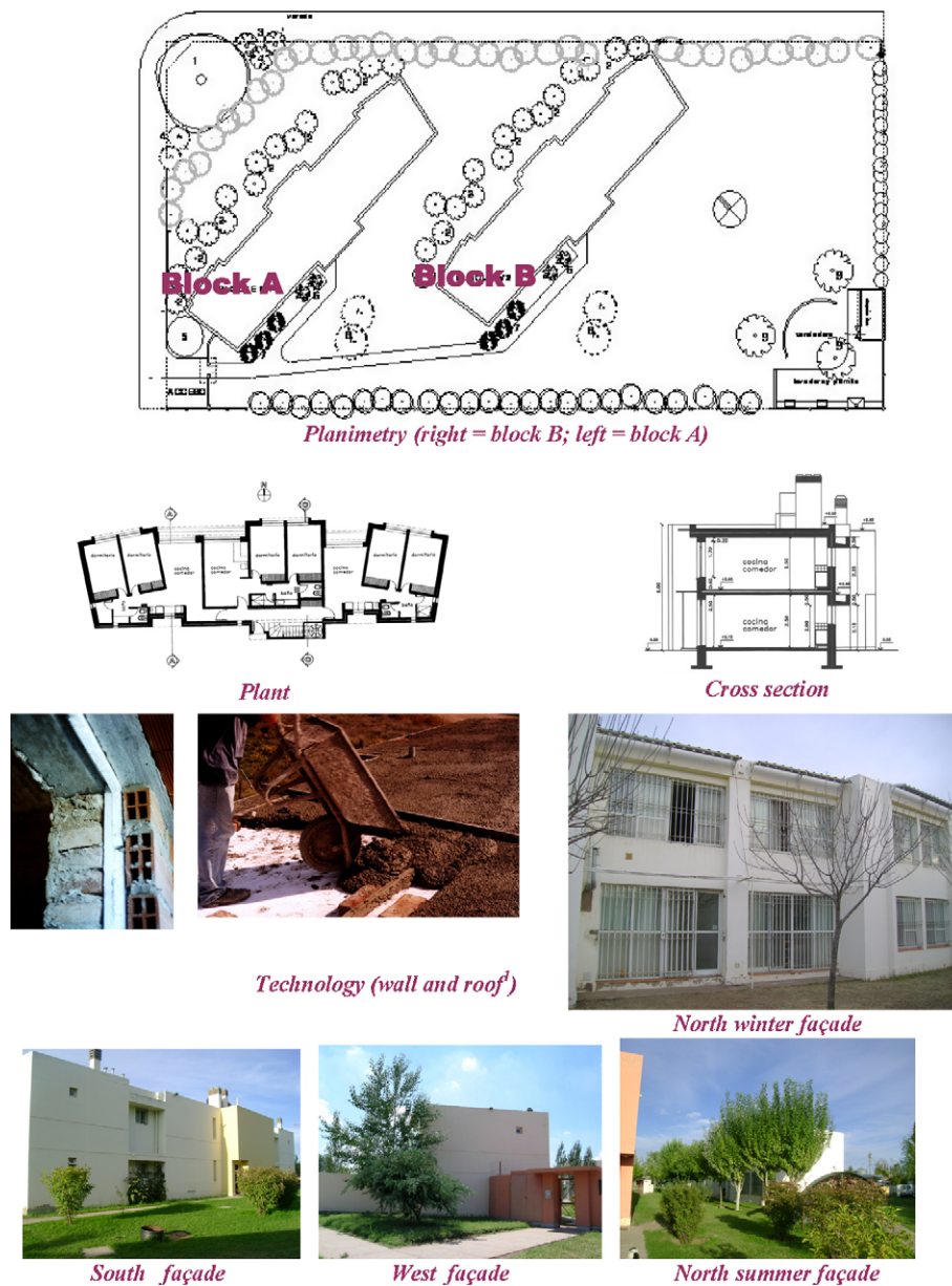
Fig. 2. Building's pictures. (1) The external walls have three layers: an inner 180 mm brick wall to provide inner thermal mass, a 50 mm thermal insulation layer, and an external ceramic wall with concrete to protect the insulation layer. Roofs were insulated with a 70 mm polystyrene sheet and a light subfloor with a waterproof layer. Hermetic aluminium frames and double glazing of windows allow to reduce heat losses and to regulate natural ventilation and daylighting. Overheating is reduced by eaves and black-out curtains.
