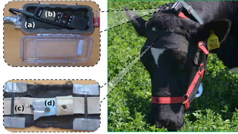
Figure 5: Box located on the cow's neck: (a) microphone plug-in and (b) recording device. Internal view of (c) the headband and (d) the microphone protected by a rubber foam on the cow's forehead.
