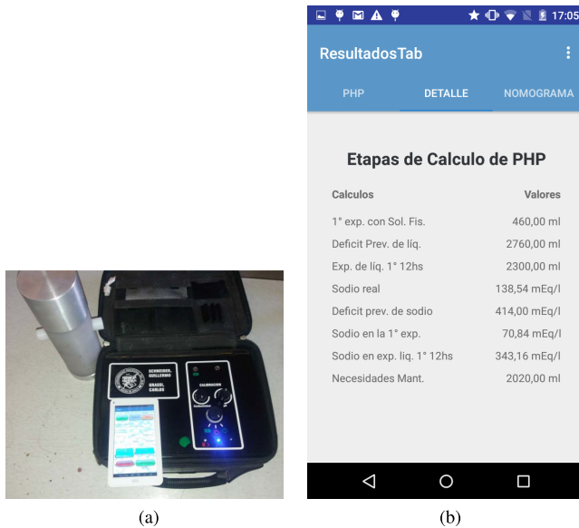
Fig. 1. Examples of projects finished with this methodology. (a) Multiparametric sensor. (b) Android application for Diabetic Ketoacidosis.
