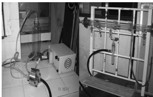
Figure 2 Standard apparatus for pervaporation.
