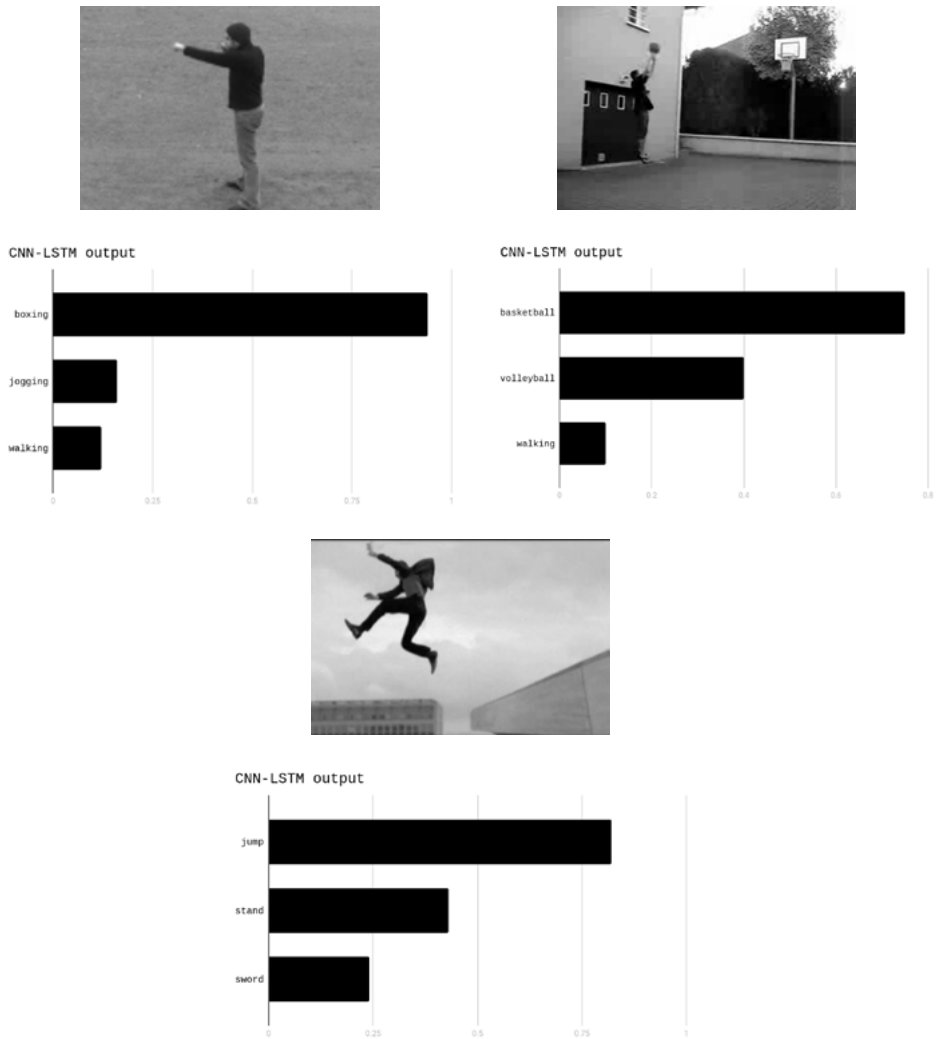
Figure 7: Top-Left: Example for KTH: This video shows a person boxing. Our system classifies it into the class “boxing”, as it reaches the score 94% (maximum). Top-Middle: Example for UCF-11: This video shows a young man throwing a ball to the basket. Our system classifies it into the class “basketball” (score 75%). Top-Right: Example for HMDB-51: This video shows a person jumping. Our system classifies it into the class “jump” (score 82%).
