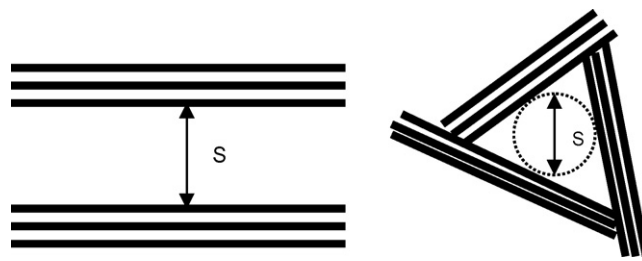
Fig. 1. Slit (left) and triangular (right) geometry pore showing how the size S is defined.
