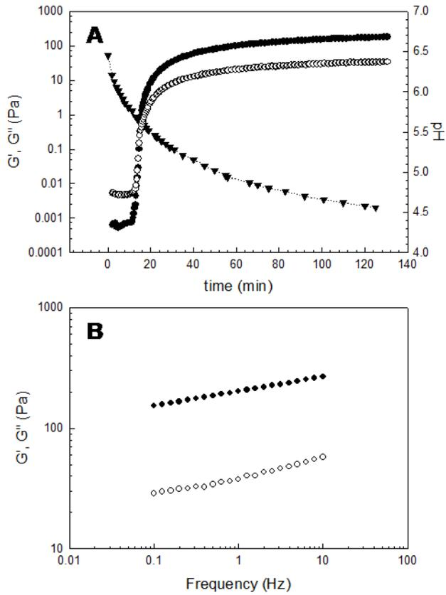
**Fig. 5.** (A) Rheological parameters  $G'$  ( $\bullet$ ) and  $G''$  ( $\circ$ ) modulus vs. time for defatted soy flour (3.0% w/w crude protein) after GDL addition (1.5% w/w) at 25°C. (B) Angular frequency dependence of  $G'$  and  $G''$  once system reached the equilibrium.
