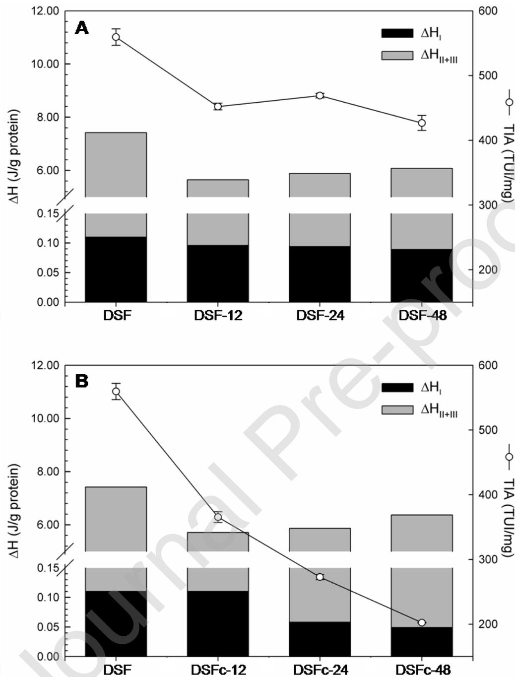
**Fig. 1.** Partial enthalpy for Peaks I and Peaks II +III ( $\Delta H_I$  and  $\Delta H_{II+III}$ , J/g protein) and total enthalpy ( $\Delta H$ , J/g protein) obtained from DSC thermograms and Trypsin Inhibitor Activity (TIA, TUI/mg) of defatted soy flour (DSF) after heat treatment at  $(60 \pm 2)^\circ\text{C}$  for 12, 24 or 48 h without (A) and with 79% relative humidity control (B): (samples
