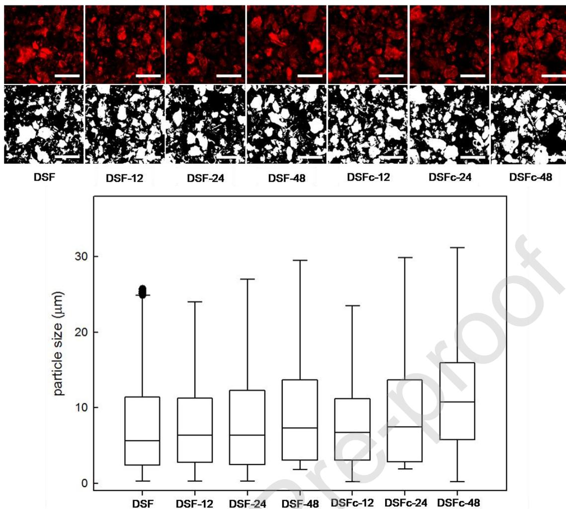
**Fig. 4.** CLSM images (on top) and their corresponded protein particle size distribution of sample dispersions (3.0% w/w crude protein) after hydrothermal treatment at 100°C for 5 min. Processed images obtained after threshold are also shown below their corresponded CLSM images. Image scale bars correspond to 50 μm.
