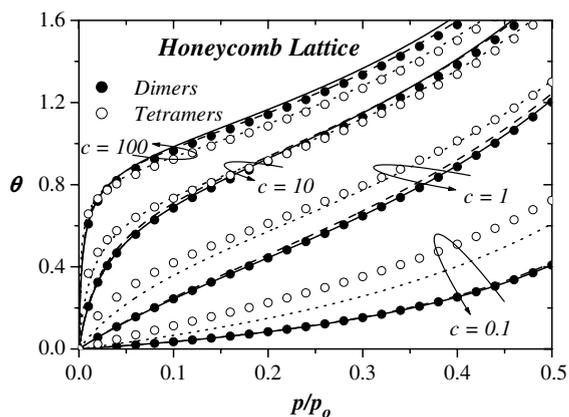
Fig. 7. Comparison between theoretical and simulated adsorption isotherms for dimers and tetramers adsorbed on honeycomb lattices with different values of the parameter  $c$ . Symbols correspond to MC simulations and lines represent theoretical results: full circles, dimers; open circles, tetramers; solid lines, data from Eq. (27); dashed lines, data from Eq. (31) (with  $k = 2$  and  $z = 3$ ); and dotted lines, data from Eq. (31) (with  $k = 4$  and  $z = 3$ ).
