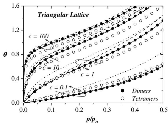
Fig. 9. Comparison between theoretical and simulated adsorption isotherms for dimers and tetramers adsorbed on triangular lattices with different values of the parameter  $c$ . Symbols correspond to MC simulations and lines represent theoretical results: full circles, dimers; open circles, tetramers; solid lines, data from Eq. (29); dashed lines, data from Eq. (31) (with  $k = 2$  and  $z = 6$ ); and dotted lines, data from Eq. (31) (with  $k = 4$  and  $z = 6$ ).
