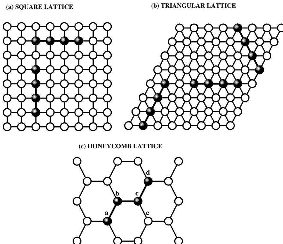
Fig. 1. Linear tetramers adsorbed on (a) square, (b) triangular and (c) honeycomb lattices. Full and empty circles represent tetramer units and empty sites, respectively.
