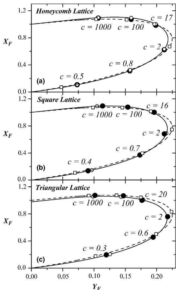
Fig. 11. Coordinates of the point of inflection (being  $X_F$  and  $Y_F$  coverage and relative pressure, respectively) for adsorption isotherms of dimers with different connectivities. Each symbol in a given curve corresponds to a determined value of  $c$ , which is indicated in the figure. Solid and dashed lines correspond to OB model and EA model, respectively, and full circles represent MC simulations results.
