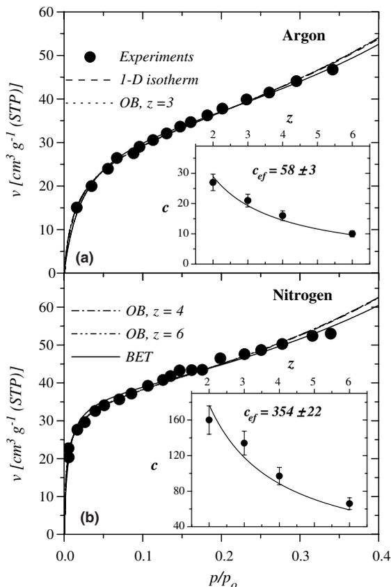
Fig. 13. Fitting of experimental adsorption isotherms of the systems Ar [part (a)] and N<sub>2</sub> [part (b)] on nonporous silica [3], through isotherms of dimers on 1-D [Eq. (23)] and 2-D [Eqs. (27)–(29)]. The resulting values of the parameters  $c$  and monolayer volume  $v_m$  are shown in Table 1 along with the ones arising from fitting with the BET model. Insets: (a) [(b)] Theoretical correlation of  $c(z)$  (as indicated in the text) for Ar [N<sub>2</sub>] on nonporous silica.
