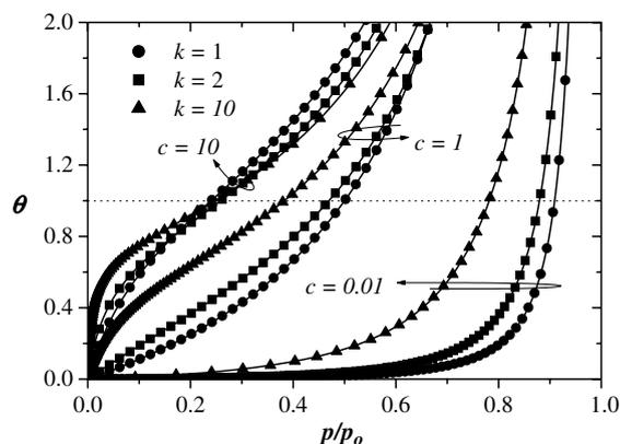
Fig. 2. Adsorption isotherms for  $k$ -mers on one-dimensional lattices and different values of the parameter  $c$  (as indicated). Solid lines and symbols represent theoretical and simulation results, respectively.
