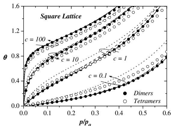
Fig. 8. Comparison between theoretical and simulated adsorption isotherms for dimers and tetramers adsorbed on square lattices with different values of the parameter  $c$ . Symbols correspond to MC simulations and lines represent theoretical results: full circles, dimers; open circles, tetramers; solid lines, data from Eq. (28); dashed lines, data from Eq. (31) (with  $k = 2$  and  $z = 4$ ); and dotted lines, data from Eq. (31) (with  $k = 4$  and  $z = 4$ ).
