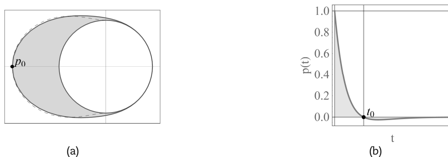
Fig. 2. Assumed pressure distribution in space and time. (a) Circumferential distribution computed from eq. (1) (solid line) and \cos^2(\theta) (dashed line); and (b) maximum pressure variation in time.
